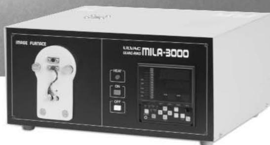
Anneal your small samples faster and with better control using the programmable MILA-3000 tabletop furnace. Ulvac's Mini-Lamp Annealing System can rapidly heat and cool samples with its infrared gold image furnace, providing precision high temperature control, clean heating and versatile atmosphere selection.
